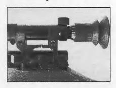
Type 89 scope mounts on a side-rail riveted to the left side of the "Para" SKS receiver. This 2 3/4 power scope weighs only 5 1/4 ounces and does not block the iron sights, but is mounted too high for a proper cheek weld.
